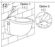
Fill the gap with white cement or glass cement.
