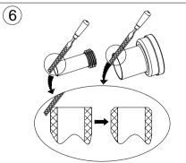
Polish the cut edges surface to get chamfer angle and deburring as per drawing.
