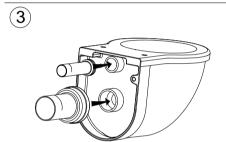
Apply lubricant on the rubber washers of the straight tube and connecting pipe, then insert them into ceramic holes.
