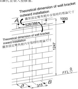
Dimension "a" according to the practical location of flushing pipe. *Note:* Above drillings are theoretical dimensions of frame mounting. Please follow the practical location of frame.
