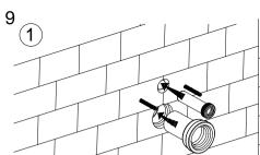
Fully insert the straight tube into the cistern flushing outlet and then connecting pipe into discharging outlet.
