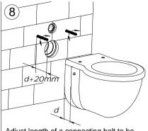
Adjust length of a connecting bolt to be  $\mbox{\bf d+20}\mbox{mm}$
