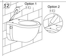
Fill the gap with white cement or glass cement. 用白水泥或玻璃膠將縫隙處補平
