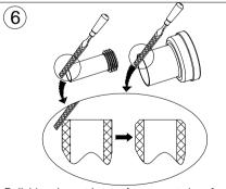
Polishing the cutting surface to get chamfer angle and as per drawing and deburring.
