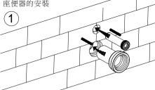
Fully insert the straight tube into the cistern flushing outlet and then connecting pipe into discharging outlet.
