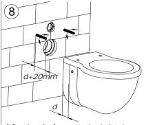
Adjust length of a connecting bolt to be d+20 mm
