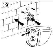
Firstly insert connecting pipe into discharging outlet and straight tube into ceramic hole.
