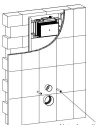
Note: According to actual size of toilet, select bolt hole size in 180mm or 230mm.
