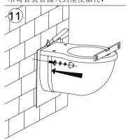
Screw the bowl and remove the extra pad. 將座便器鎖定並沿著座便器外形將多出襯墊去除
