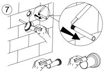
Cut the protection sleeve outside of the wall with a knife.
