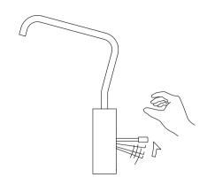
\* 6777-G1-80CP Drinking Faucet (HOT) has been designed with protective device. The faucet will continuously flow by holding the handle; it will stop flowing and lock again as letting go the handle. 6777-G1 is suitable for connecting with hot water outlet device. 型號6777-G1有保護裝置,須持續按壓方可連續出水,放手後將會自動關閉,並上鎖。適合用於熱水場合。
