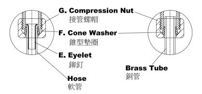
\* Connect hose or brass tube with **Cone Washer**, **Compression Nut**, and **Eyelet** as fig. shows.
