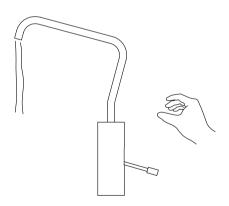
\* 6777-G0-80CP Drinking Faucet (COLD) will keep flowing as operating, and it will be closed by restoring the handle by hand. 6777-G0 is suitable for connecting with non-hot water outlet device.
