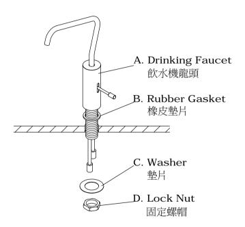
\* Slide **Rubber Gasket** onto the **Threaded Shank**, and then insert **Threaded Shank** down trough deck. Assemble **Washer** and **Lock Nut** onto **Threaded Shank**, and then tighten the **Lock Nut**.
