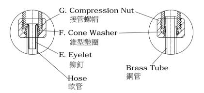
\* Connect hose or brass tube with **Cone Washer**, **Compression Nut**, and **Eyelet** as fig. shows.
