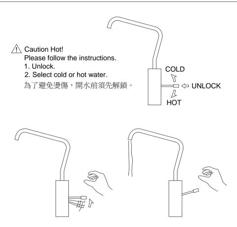
\* Hot water operation has been designed with protective device. The faucet will continuously flow by holding the handle; it will stop flowing and lock again as letting go the handle..
