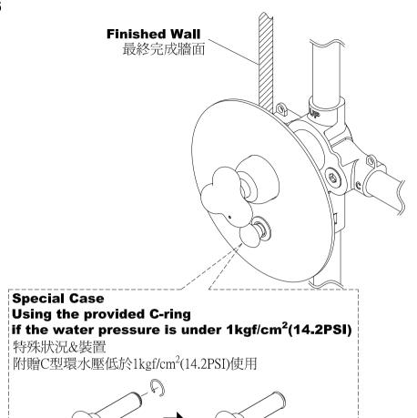
\* If the Water Pressure is too low to function the diverter, please use the provided **C-ring** for manual control.
