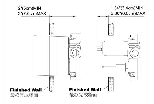
\* Connect hot and cold supplies pipes to the valve body and meantime install outlet water ways, and keep the distance between 2"(5cm) minmum and 3"(7.6cm) maximum from the finished wall; or keep the distance be 1.34"(3.4cm) to 2.36"(6.0cm) between top of cartridge and **Finished Wall** for necessary conditions.
