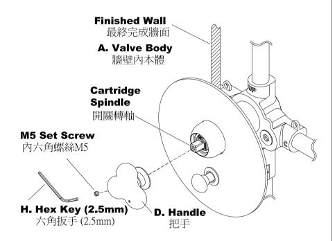
\*Fix the **Handle** with **M5 Set Screw** to the **Cartridge Spindle** by **Hex Key**.
