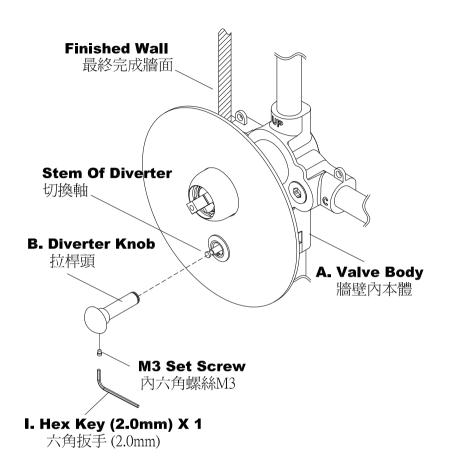
\*Fix the **Diverter Knob** with **M3 Set Screw** to the **Stem Of Diverter** by **Hex Key**.
