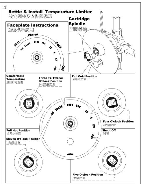
\*Before install the **HANDLE**, please rotate the **Cartridge Spindle** to the position of comfortable temperature.
