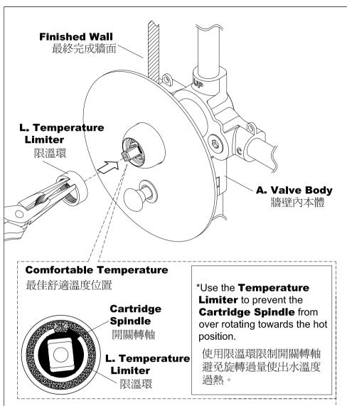
\*Rotate the **Cartridge Spindle** to the position of comfortable temperature and then install the **Temperature Limiter** into the cartridge.
